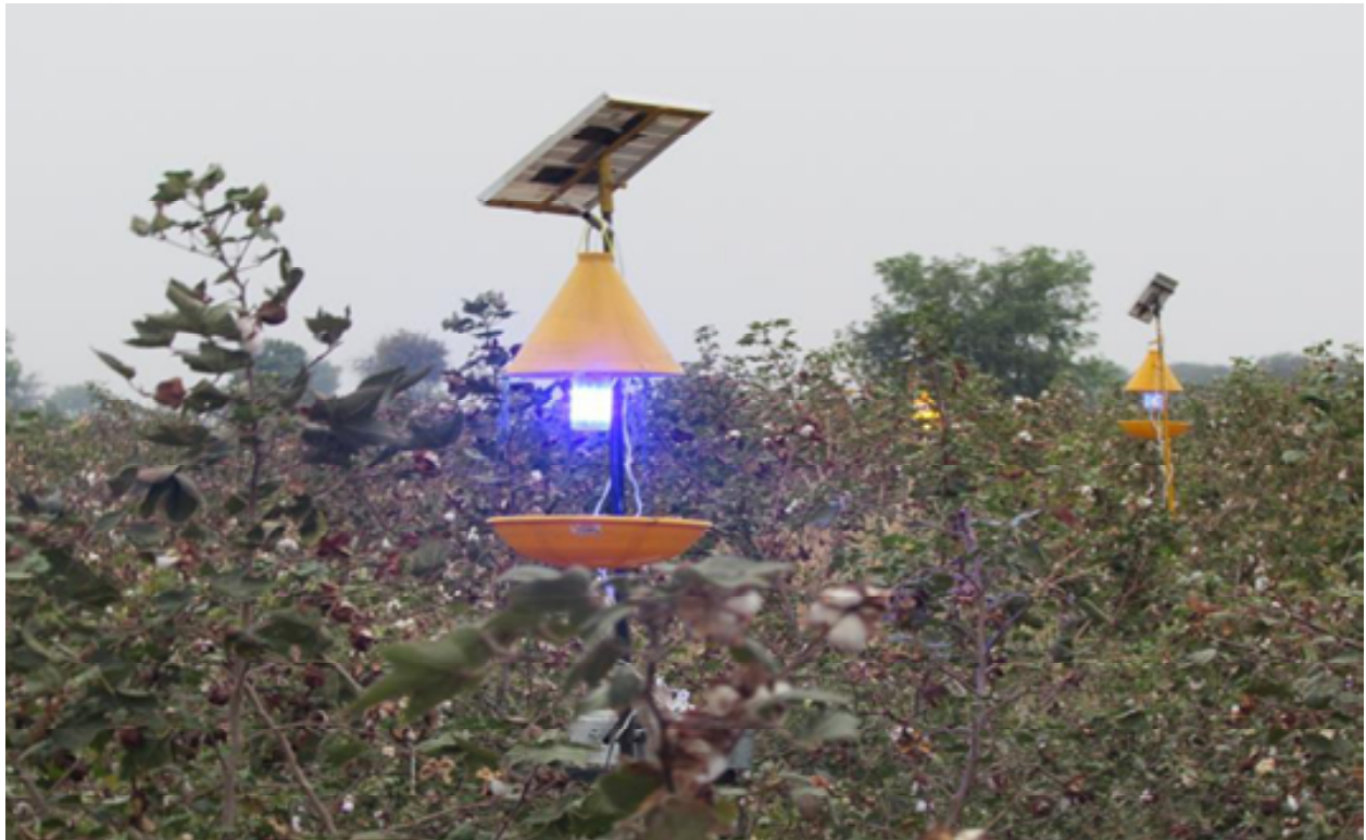
figg. 3 Field performance of solar photovoltaic insect light trap
